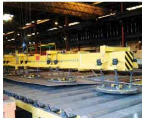
Large-sized vacuum beam with a peak load of 12 t, equipped with level compensation for steel sheets with a high ripple content
