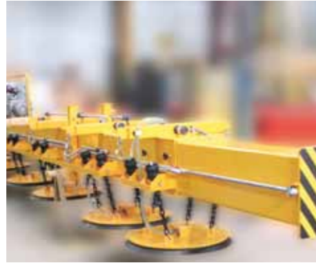
Large vacuum beam with a maximum load capacity of 12 t for heavy steel plates or sheets
