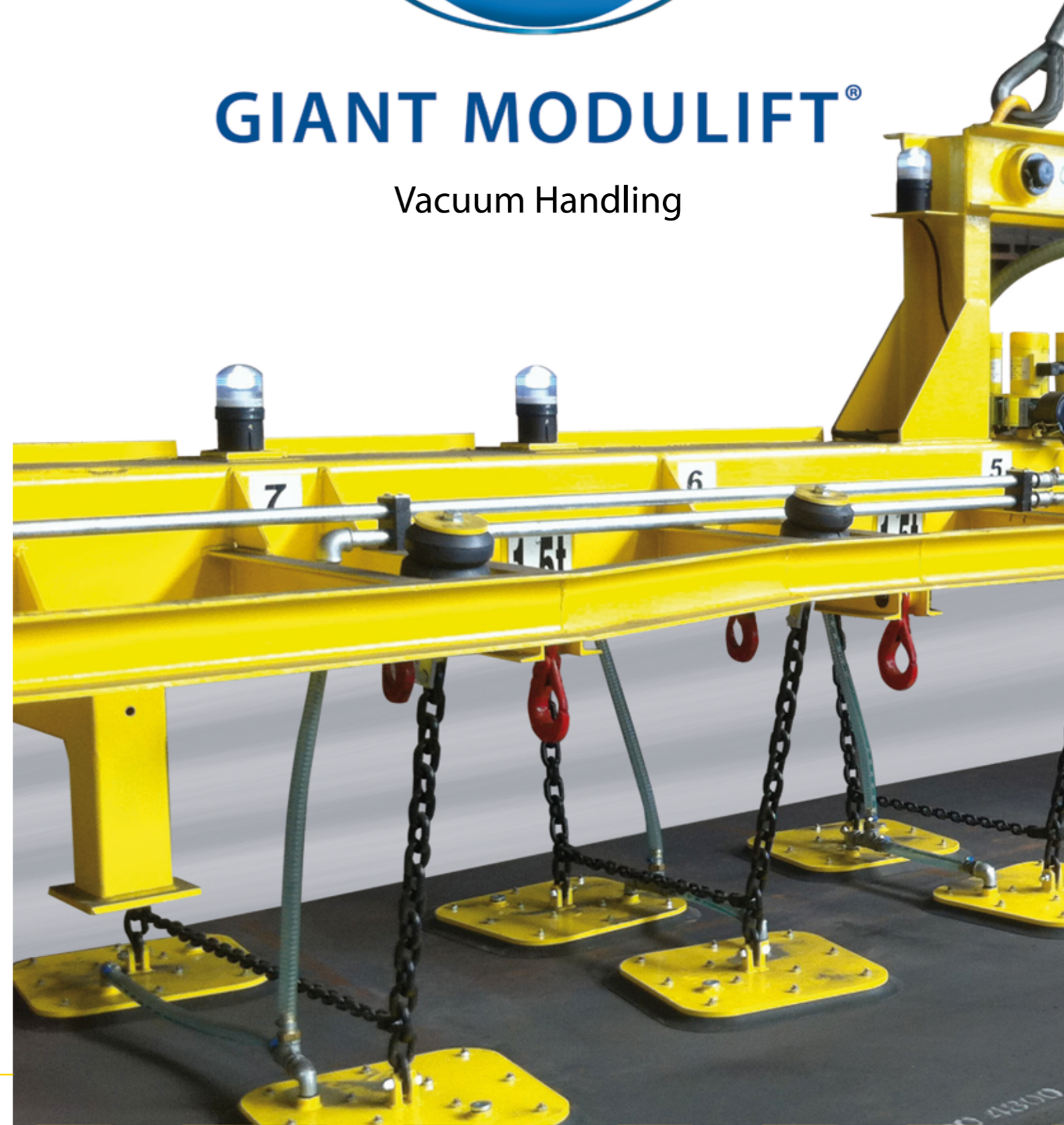
Vacuum system equipped with a 1400 x 1400 mm gasket and a peak load of 10 t for horizontal or vertical stocking of heavy steel plates or sheets
