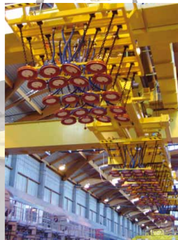
80 suction cups with diameter of 310 mm
