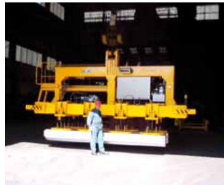
Handling system for aluminum blocks with a maximum load of 10 t
