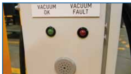
Audiovisual alarm for current industrial environment. Noise: 50dB buzzer
