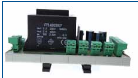
E-card fitted in each Modulift vacuum lifter (advantages: reliability, compactness)
