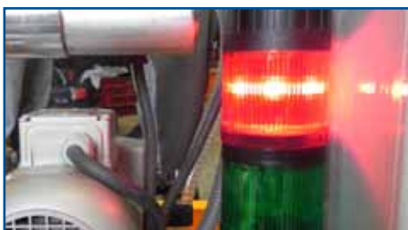
Audiovisual alarm for rough industrial environments. Noise: 80dB siren
