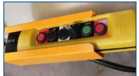
Pilot control: solenoid valves with push button control box
