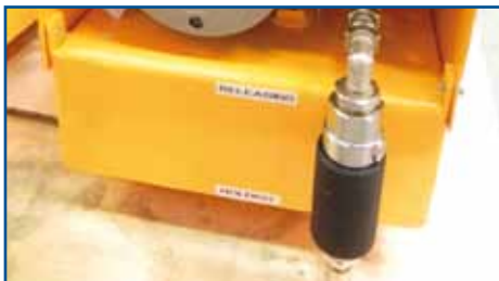
Manual control : secure sliding sleeve valve
